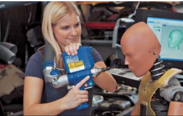
Bethany Koetje, MS '08, digitizes a crash test dummy at the National Crash Analysis Center.
